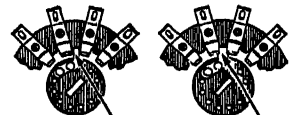
WIDTH OF ROTOR TOOTH LESS THAN DISTANCE BETWEEN CONTACT CLIPS NON-SHORTING TYPE WIDTH OF ROTOR TOOTH GREATER THAN DISTANCE BETWEEN CONTACT CLIPS SHORTING TYPE
